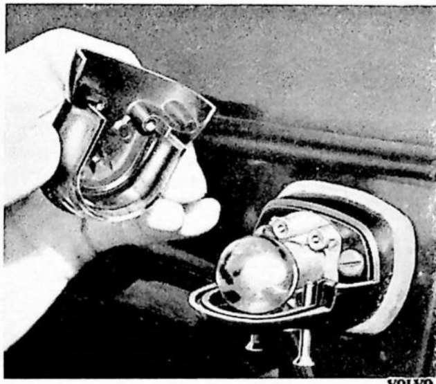
Fig. 34. Traffic indicator for P 44403/4 Chassis Nos. 28005—37004 (late prod.) and chassis Nos. 37005—68955.
