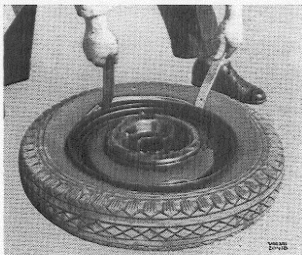
Fig. 24. Fitting the tyre, upper part.
