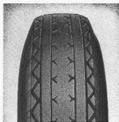
Fig. 6. Tyre wear, air pressure too high.
