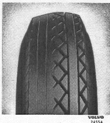
Fig. 8. Tyre wear, faulty camber.
