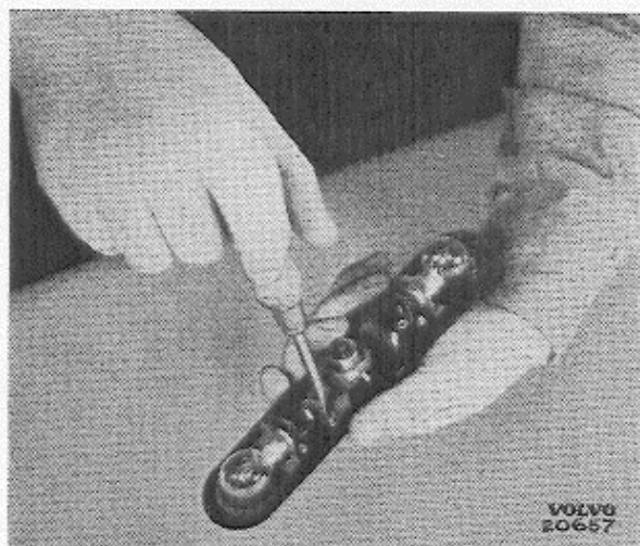
Fig. 33. Traffic indicator (Roof mounted type).
