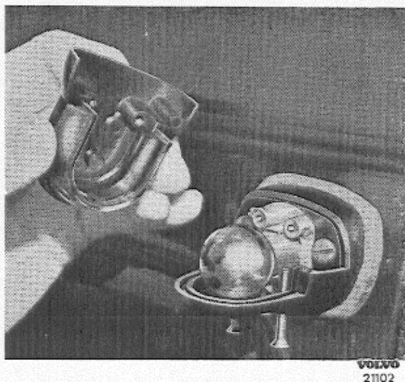
Fig. 34. Traffic indicator for P 44403/4 Chassis Nos. 28005—37004 (late prod.) and chassis Nos. 37005—68955.
