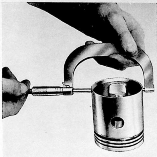
Fig. 35. Measuring a piston.
