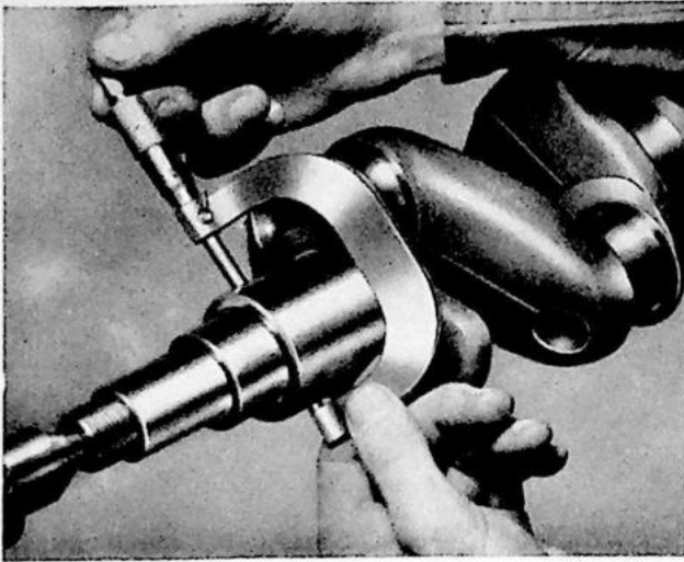
Fig. 33. Gauging a bearing journal.
