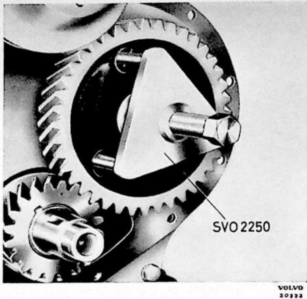
Fig. 28. Removing the camshaft gear.
