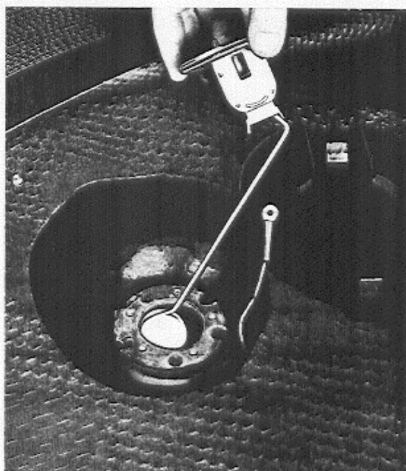
Fig. 11. Removing the tank fitting
