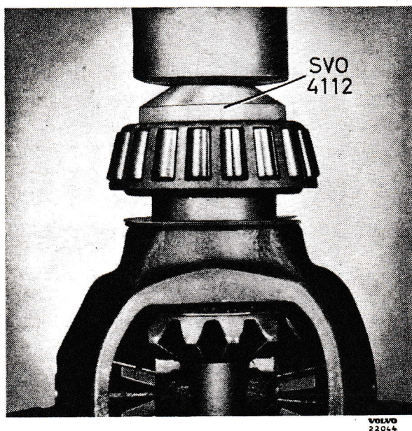
Fig. 18. Fitting the differential case bearings.
