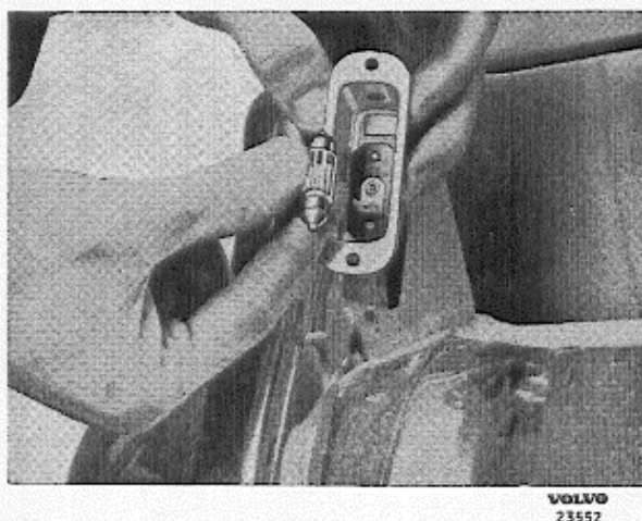
Fig. 21. Removing the bulb.
