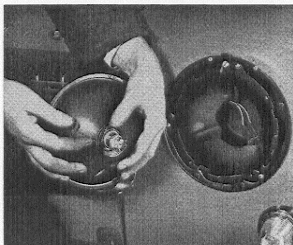
Fig. 69. Removing the bulb holder spring.
