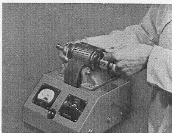
Fig. 44. Testing the rotor.
