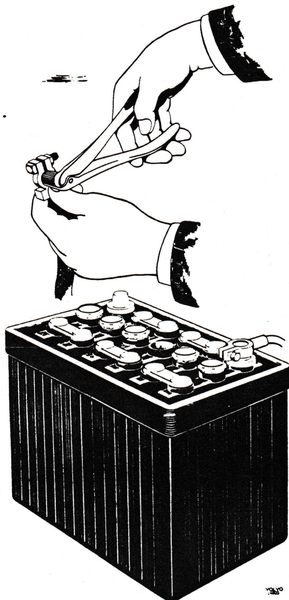
Fig. 15. Cleaning battery cable terminal
