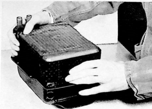
Fig. 22. Fitting the cell system
