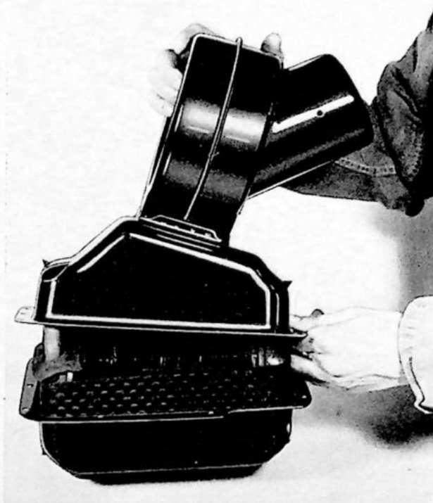
Fig. 23. Assembling the heater
