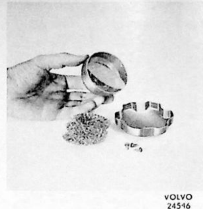
Fig. 12. Oil filler cap.
