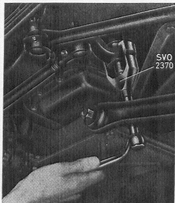
Fig. 28. Removing pitman arm
