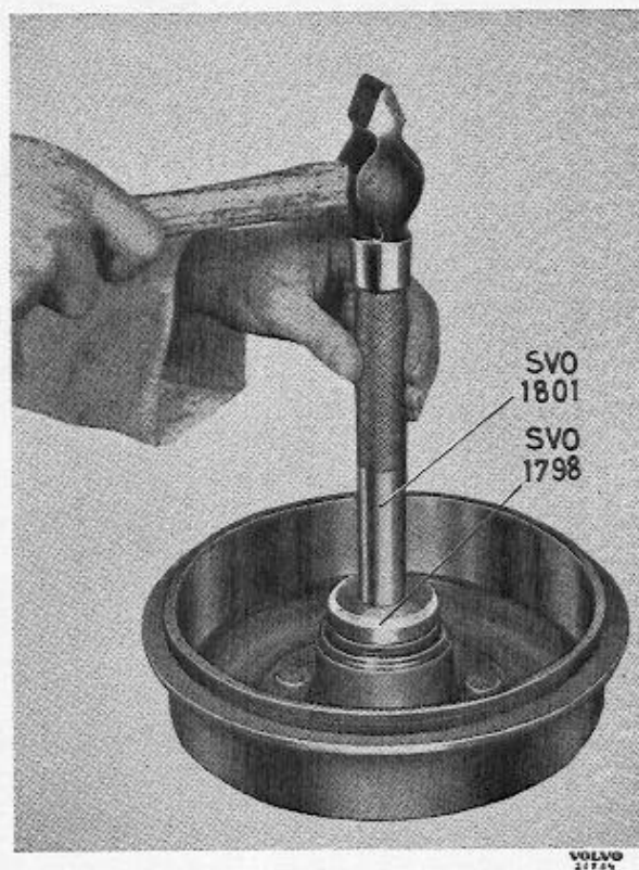
Fig. 9. Fitting the seal ring.
