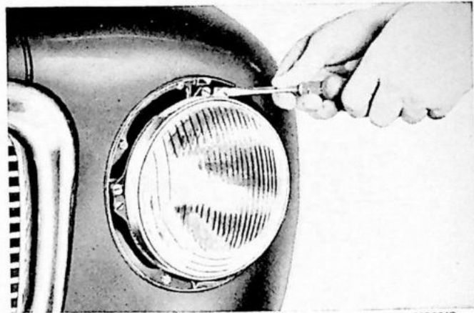
Fig. 12. Removing retainer ring.
