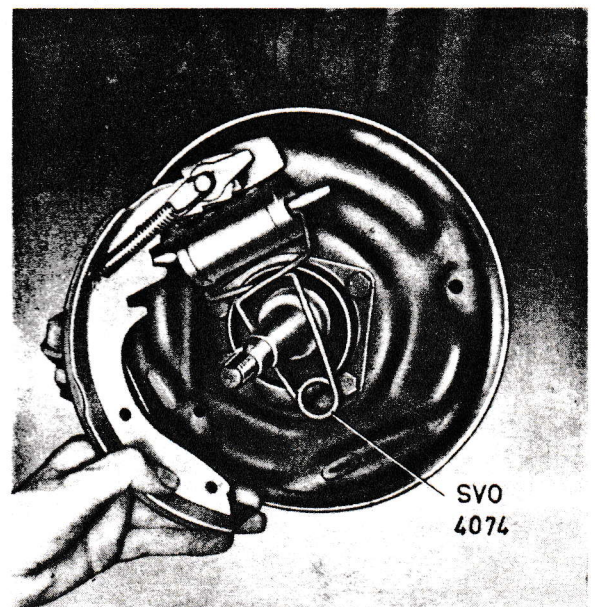
Fig. 20. Fitting the brake shoe.
