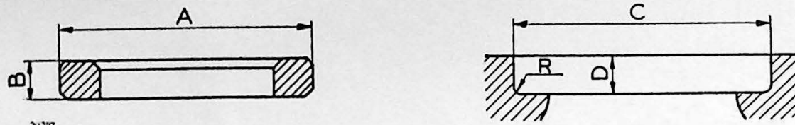
Fig. 3. Outline of valve seats and positions.
